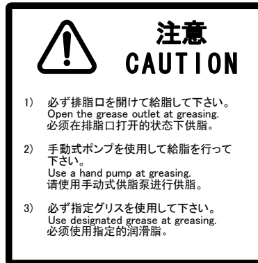
Fig. 4 (a) Greasing and degreasing label
