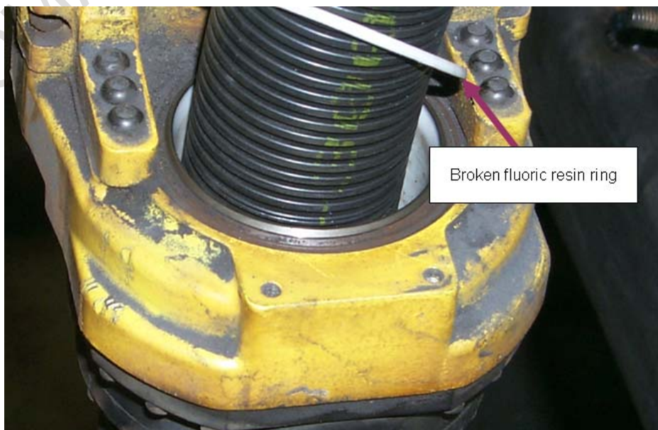
Fig .1.2.4 (b) Failure of the fluoric resin ring
