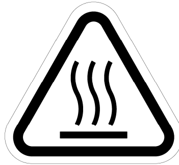
Fig. 4 (c) High-temperature warning label
