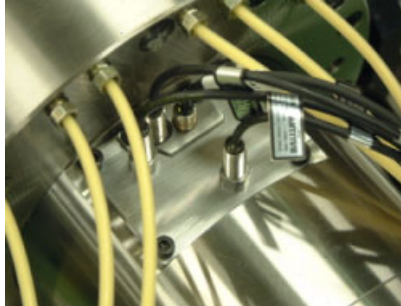
Detection switches : 4 each (20000min -1 , installed)
