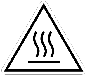
Heat caution label (compliance with the IEC standard)
