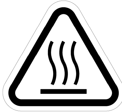
Fig. 10 (c) High-temperature warning label
